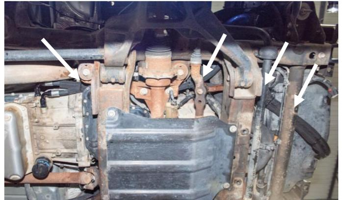
The short length hose is routed from the transmission "TO COOLER" to the bottom-side radiator fitting. The 45 degree fitting is utilized on the radiator side, aligned slightly downward and toward the center of the chassis
