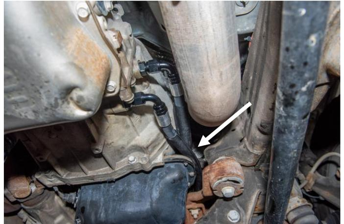
Route the long and short length lines over the main chassis members and suspension anti-roll bar.
