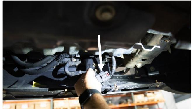
**STEP 7:** Remove the lower supports for the front bumper from the left and right sides of the vehicle.
