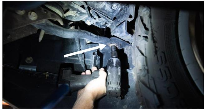
**STEP 8:** Remove the front bumper assembly to provide for clear access to the transmission oil cooler.
