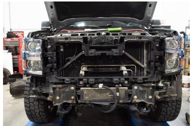
**STEP 9:** Remove the lower engine shroud.
