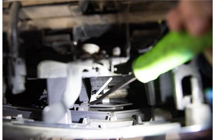
**STEP 5:** Remove the bumper by removing the upper retaining bolts with an 18mm socket.
