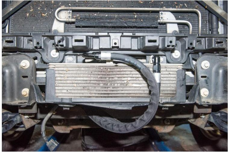
Route the medium and long length lines over the top of the chassis cross-tube together.
