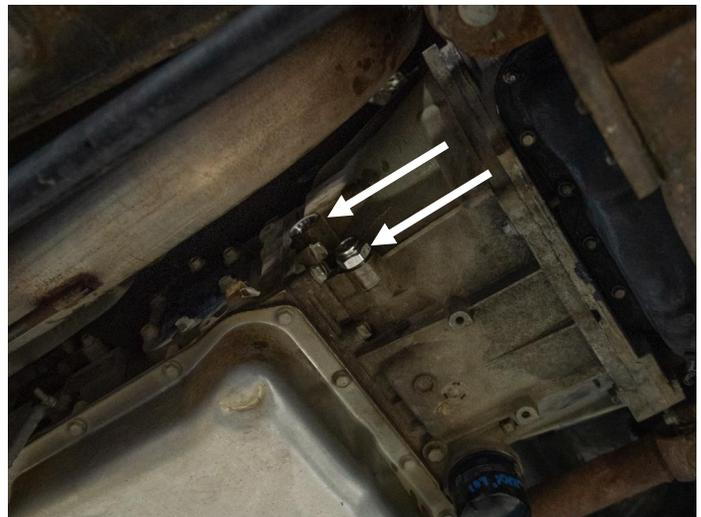
**STEP 12:** With the OE transmission lines removed from the truck, use a 1 1/8" back up wrench and 1 1/4" socket or wrench to remove the factory fittings from each side of the transmission cooler.
